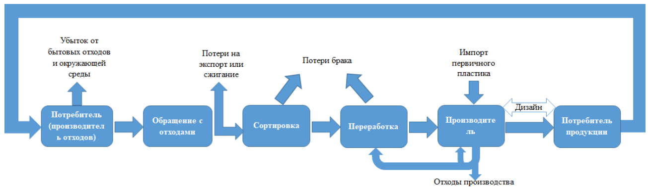
Figure 1. Value chain for plastic waste recycling
