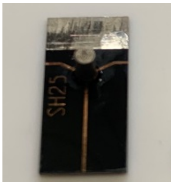
Fig. 5 - Prototype of Ka-range Y-circulator and its electrical parameters
